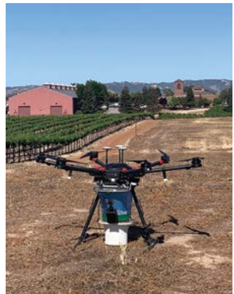
At Robert Hall Winery, drones transport predatory insects to eradicate mealybug populations.
