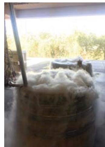
Martin Mackenzie uses dry ice to cool the temperature during ferments in French oak puncheons.
